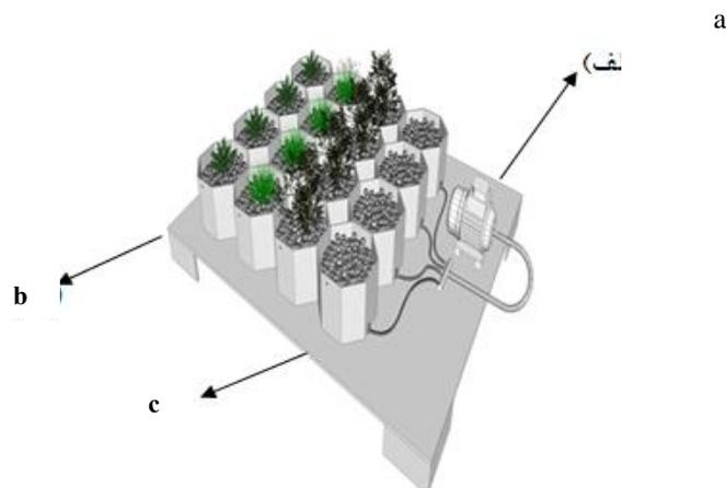
**Figure 1. Used pilot in research a) air pump b) reactors with plant c) control reactor**
