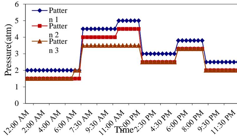
Figure 2.3 patterns applied on the modulated PRV
