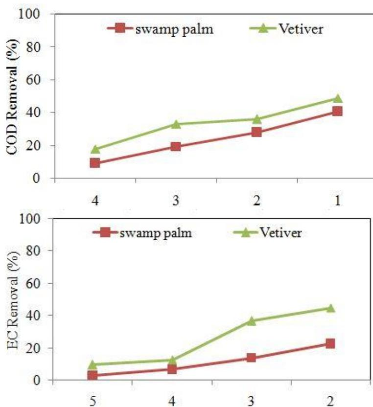
Comparison of COD and Electrical Conductivity Removal
