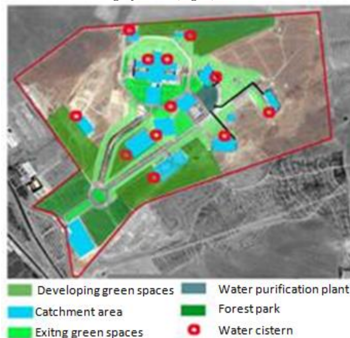
Fig. 1. Strategic design of campus green space based on rain harvest and reuse of gray water
